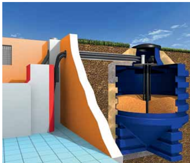
Plate 8: Below-ground silo made from synthetic materials, discharge from below
