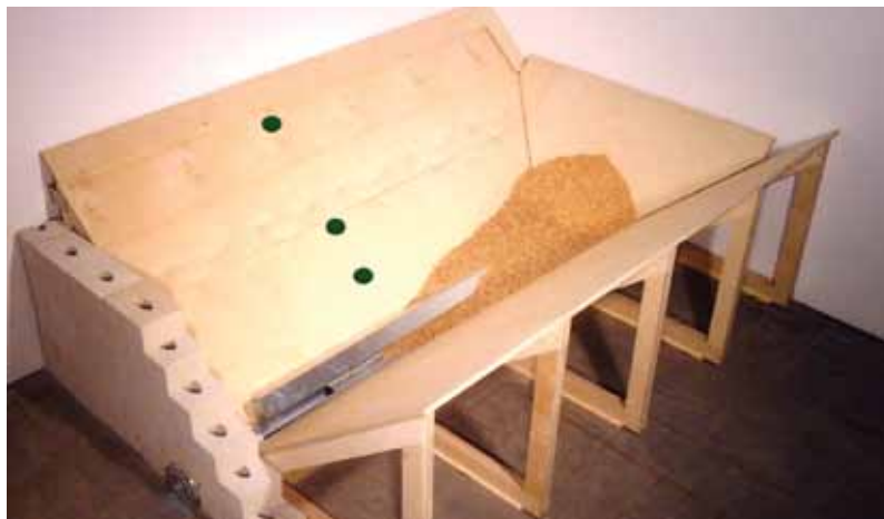
Plate 25 Pressure sensor for the filling status in an inclined bottom
